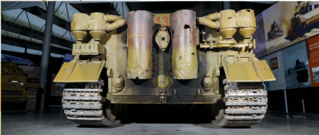
The Tiger had a complex exhaust system on its rear to increase power
